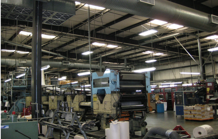
Casey Printing's production area equipped with T-8 fluorescent lamps
